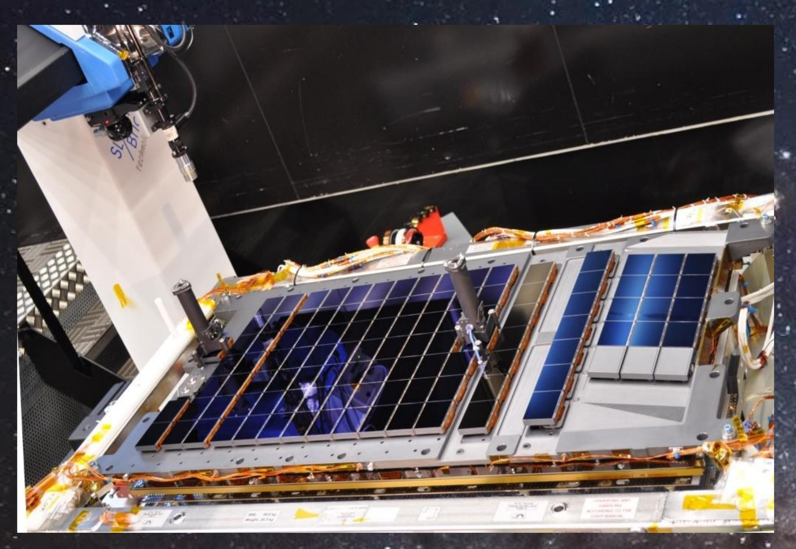
Figure 1: Gaia Focal Plane Assembly with all 106 Charge-Coupled Devices in place prior to integration into the science payload module. Picture credit: ESA / Airbus DS (formerly Astrium), October 2011.
