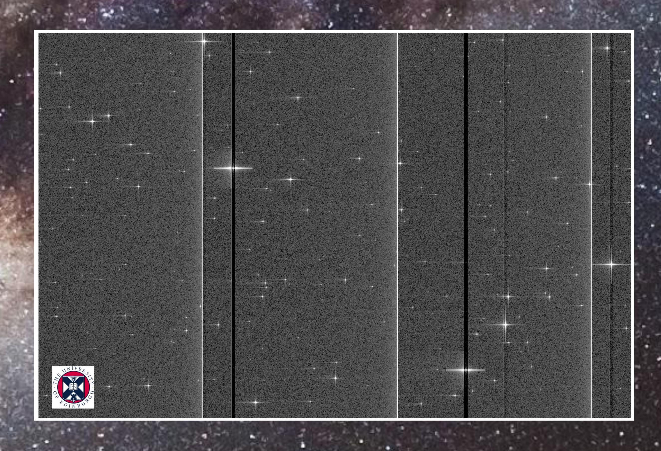
Figure 2: simulated image of the sky as seen by Gaia. Large-scale vertical and horizontal stripes are electronic instrumental effects resulting from the operating mode of the CCDs. The Edinburgh University team is responsible for monitoring, analysing and removing these effects in the Gaia data. This key step must be done before the astronomical information can be extracted from the image data. Picture credit: Edinburgh University IfA "VitrualScan" Gaia simulator
