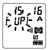
Set the "D"-Dial to the "UP" position. When you press the shutter button "Half-way" the camera will set the focus and exposure. As you press the shutter button further, the mirror will move up and the exposure value will be memorized. Remove your finger from the shutter button and lightly press.
