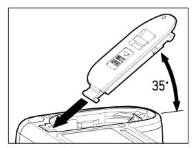
It is possible to remove battery cover, if it is tilted around 35 °. If this part comes off during opening or closing the cover, please insert cover as shown in the illustration.
