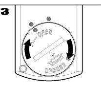
Check controller operation after replacing the battery.
