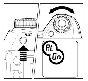
Press *FUNC* button six times (press and hold the button at the sixth depression), *RL* mark will be displayed on the top LCD. Do not release the *FUNC* button.
