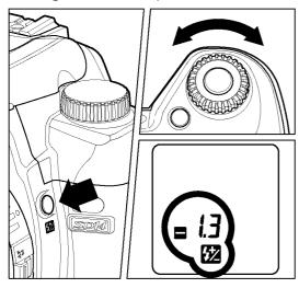
While pressing the **122** button, turn the "C"-dial to set the compensation amount.
