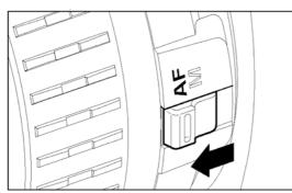
Set the AF/MF switch on the lens to the AF position. (P.46)
