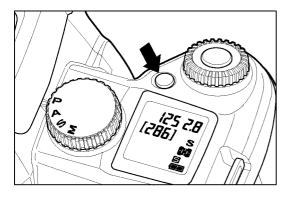
Pressing the "Top LCD Illumination Button" activates the orange color LCD illuminator, allowing the Top LCD display to be read in the dark.
