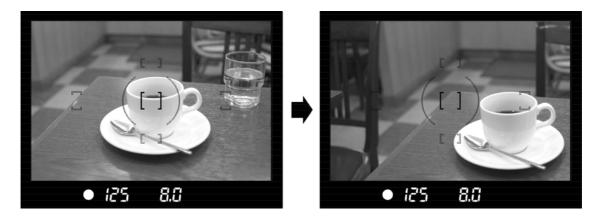
Focus Lock can be used with **S** (single AF mode) only. The AF cannot be locked in **G** (continuous AF mode).
