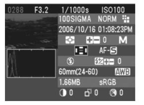
This histogram shows that the higher pixel values are never used in the image, indicating that the image is underexposed, and therefore will appear dark. In general, when the histogram is higher on the left side, the image is mostly composed of dark pixels, causing it to appear dark—either because the image is underexposed or because it is a dark scene such as night shot or sunset.
