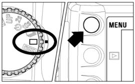
**T** Press the **MENU** button on the back of the camera to display the Camera Set-up Menu. (See **P.104**)
