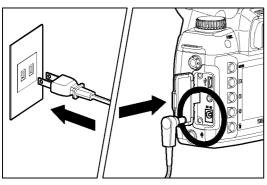
Connect the AC adapter to the camera and plug it into a wall socket. (**P.23**)
