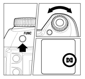
While pressing the **FUNC** button, rotate the "C"-dial to select the desired metering mode and display it on the LCD panel. Releasing the metering button sets the selected metering mode.
