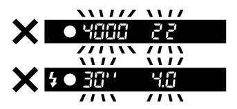
If the subject is too bright or dark, both shutter speed and aperture value indicators will blink and will show the limit values. If you take a picture with these settings, the picture will be overexposed or underexposed.
