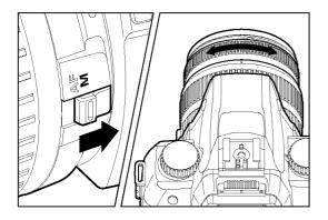
Set the focus mode switch, on the lens to the **M** position (AF mode mark will disappear from the LCD panel).
