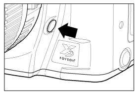
However, by pressing the depth-of-field preview button, the aperture can be closed down to the selected shooting aperture before the picture is taken, enabling you to check depth of field through the viewfinder before shooting.
