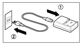
Connect the power cable to the charger and insert the plug into the wall outlet.
