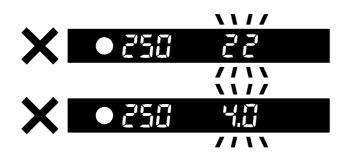
If the appropriate aperture value is beyond the range of the lens in use, due to the subject being too bright or too dark, the aperture value indicator will blink. If the subject is too bright, set the shutter speed to a faster one, or if the subject is too dark, set the shutter speed to a slower one, until the indicator stops blinking.
