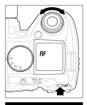
Press ⊡ button and select the desired AF point by rotating the "C"-dial displayed in the viewfinder.
