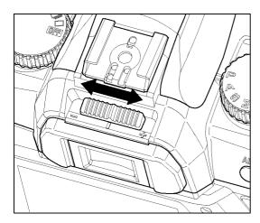
While looking through the viewfinder, slide the diopter adjuster to the left or to the right, until the image appears sharp on the focus screen.
