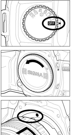
Make sure to turn the "D"-Dial to **OFF** position (Power Off position)
