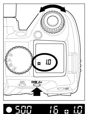
While pressing **BA***v* button, turn the "C"-dial to set the desired compensation value. Then, release the Exposure Compensation button.
