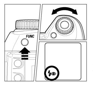
Press the *FUNC* button 3 times and hold. The LCD panel will display the flash mark ( 4 ). Do not release the *FUNC* button.
