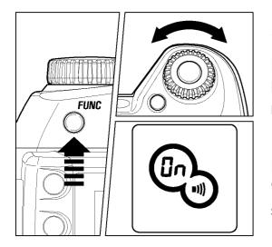
Press the **FUNC** button 5 times and hold. The LCD panel will show the **III**) symbol. Do not release the **FUNC** button.
