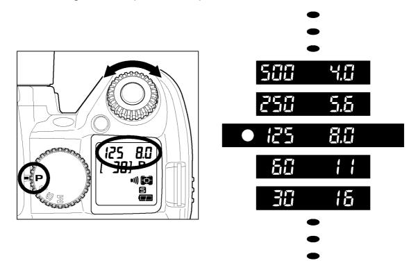
It will be canceled automatically, after taking the picture. A program shift cannot be performed while using the flash.
