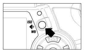
Press the *Iso* . button on the back of the camera to open the Image Setting Menu.
